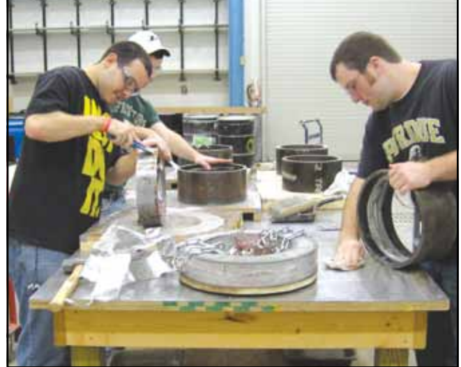
Purdue student Paul Imbrock (top) performs ASR (Alkali Silica Reaction) testing. ASR is a reaction that occurs with sand or rocks and causes cracks in the concrete. Below, students help prepare ring tests, which evaluate cracking resistance.
